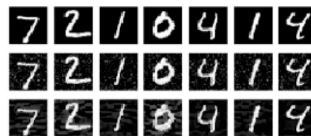
Figure 1. Examples of normal (top), noisy (middle) and adversarial (bottom) MNIST samples for a convnet. Adversarial samples were crafted via the Basic Iterative Method (Kurakin et al., 2017) and fool the model into misclassifying 100% of the time.
